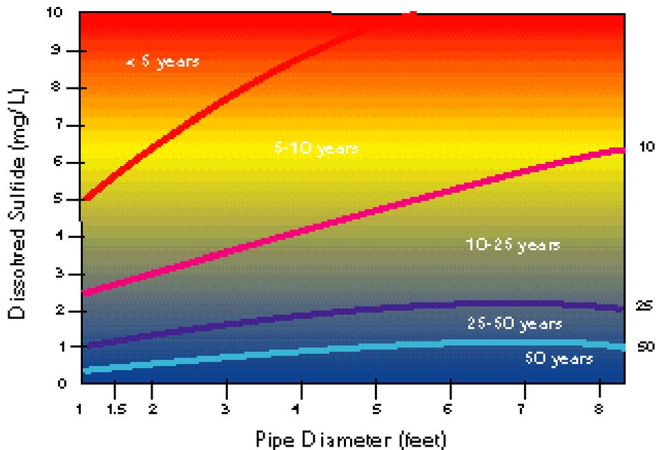
Figure 4. Effect of H<sub>2</sub>S on Concrete Pipe (American Concrete Pipe Association)
