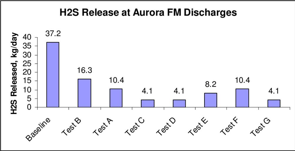
Figure 2. Gaseous H<sub>2</sub>S Released at Turbulent Aurora Forcemain Discharges
